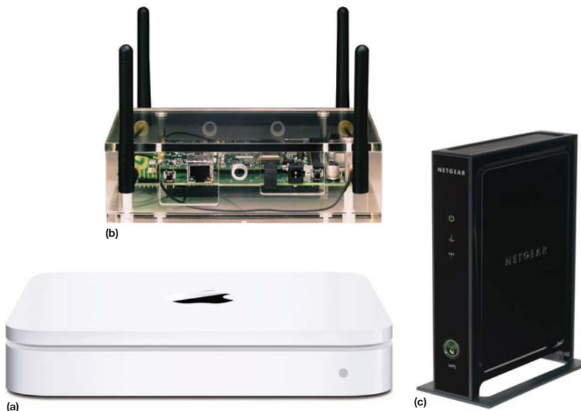
Figure 1 Apple's latest-generation Airport Extreme 802.11n router and Time Capsule router-plus-NAS integrate three-stream support, although the company doesn't explicitly promote this feature (a). Quantenna's four-stream silicon-and-antenna-array approach (b) just received its first high-volume consumer-electronics production embrace in the form of Netgear's WNHD3004 wireless bridge (c).
