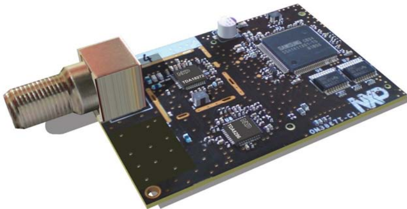
Figure 1 This NXP silicon-tuner evaluation board has provisions for shielding a metal can around the chip, but some applications may not require the can.
